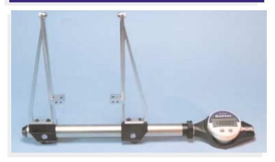
Measuring arms of length 200 mm are now available for the standard Universal Gauge. The new measuring arms can be used for both internal and external measurement and are particularly useful for deeper internal measurements or for bridging high spigots and shoulders. Extra stability is provided by a rear support strut and standard depth stops can be fitted just as for standard length measuring arms.
